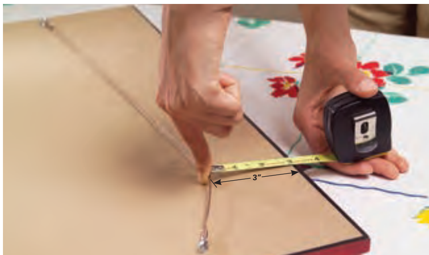
3 Leave one finger in place and measure from the wire to the top. Use this dimension and the dimension from Photo 2 to position the picture hangers.
